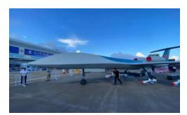
Release date: 09/29/2021 Used by: China Characteristics: endurance 18h (strike variant) or 21h (ISR variant), top speed 700 km/h, 45,000 ft. ceiling, 450 kg payload Price: \$6-8 million
