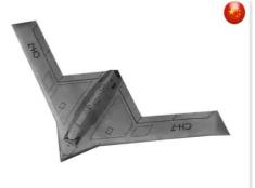
Release date: in development (estimated to be operational in late 2022) Used by: China Characteristics: 15h endurance, 2,000 km range, top speed 920 km/h, 36,000 ft. ceiling, **stealth** combat drone, **stand-off** purpose Price: (?)
